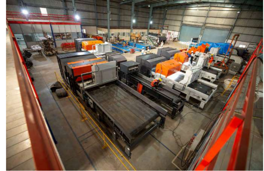
Automated material recovery facility (MRF) using Ishitva's AI-enabled waste sorting line | Image Source: Ishitva
